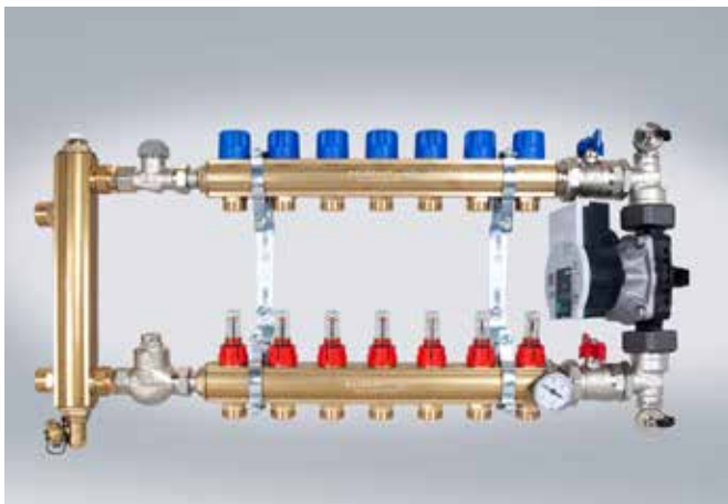
Control manifold HCM-DR with high-efficiency pump and thermoseparator, version 2.0, 2-9 heating circuits 1" IT or 10-16 heating circuits 5/4"
